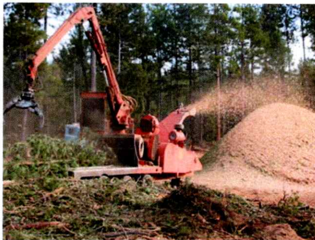
Figure 17. Removal by chipping -One method to remove slash from the site is to use high powered chippers and trucks to haul material to utilization or disposal sites.
