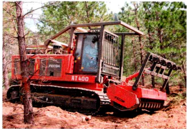
Figure 10. Front end masticator - Mastication is the preferred choice for woody residue treatment
