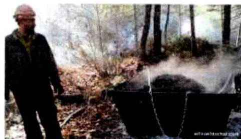
Figure 15. The Forestry Flame Cap Kiln. Designed by Wilson Biochar Associates for use in forestry to convert burn piles to biochar. Newer model will have fork pockets for lifting and unloading. .Biochar for Forest Restoration in the Western United States – 9-18-15 (rev.3-15-16)
